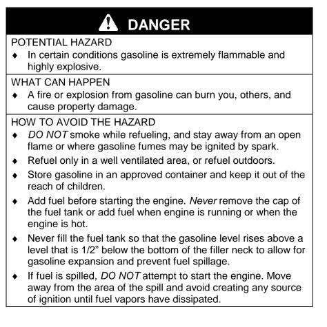
4.2.1 Fill fuel tank. For best results use only clean fresh regular grade **unleaded** gasoline with an octane rating of 87 or higher. Regular grade leaded gasoline may also be used; however, combustion chamber and cylinder head will require more frequent service. See Engine Owner's Manual.
